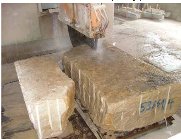
Initial processing of a limestone block
