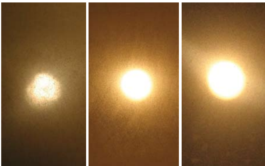
Photo No. 1. The same halogen light reflected off 3 different tiles gives 3 different levels of haze around the light. This is considered to be conventional optical hazing. There are few complaints about this type of hazing, all the tiles pass the requirements of ISO10545
