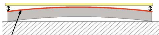
Figure 4. Schematic diagrams showing the differential movement effects observe in natural stone tiles. The upper face expansion can also occur with moisture sensitive tiles exposed to ponding rain water.
